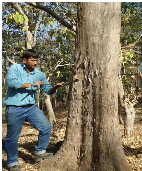
Figure 2: Core sample obtained by non-destructive methods through increment borer.
