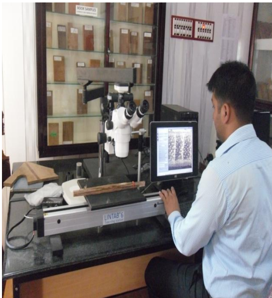
Figure 4: Measurement of tree ring width and vessel area in core sample of teak.
