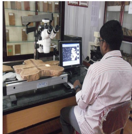
Figure 5: Measurement of tree ring width and vessel area in basal disk sample of teak
