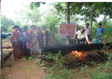
Boiling Method of Bamboo Treatment at CFLE Campus
