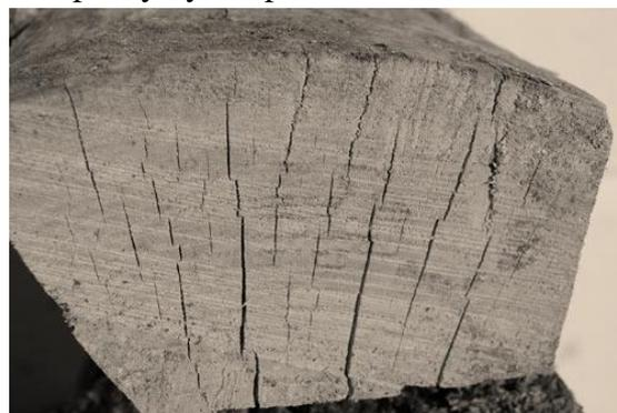
Aside from the loss of water, which takes place in seasoning, other changes occur. The bordered pits become more or less ruptured, or changed in position, so that passage of liquids through them is facilitated or retarded. Furthermore, the wood cells frequently check as well as the
