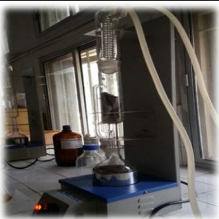
Fig.40 Extraction of crude extracts using Soxhlet Apparatus
