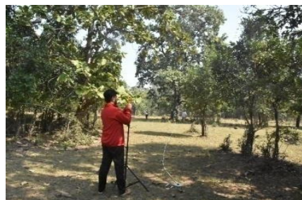
Fig.8 Measurement of tree diameter at different height segments at Bastar forest division using Basal Area Finder (BAF) Scope
