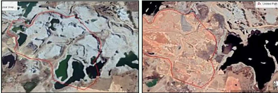
Google extract of Bellahalli quarry area (left hand side) and right hand side) Quarry after covered with soil creating a vegetation cap of 4 to 5 feet (Courtesy - BMRCL)
